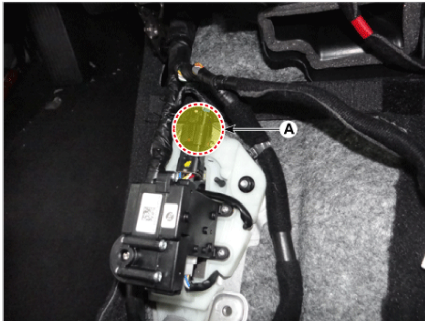
13. Disconnect the airbag control module connector (A) and wiring mounting clips.
